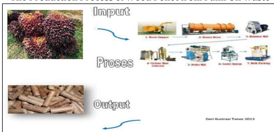
Figure 4.2 The Production Process of Wood Pellet from Palm Oil Waste
