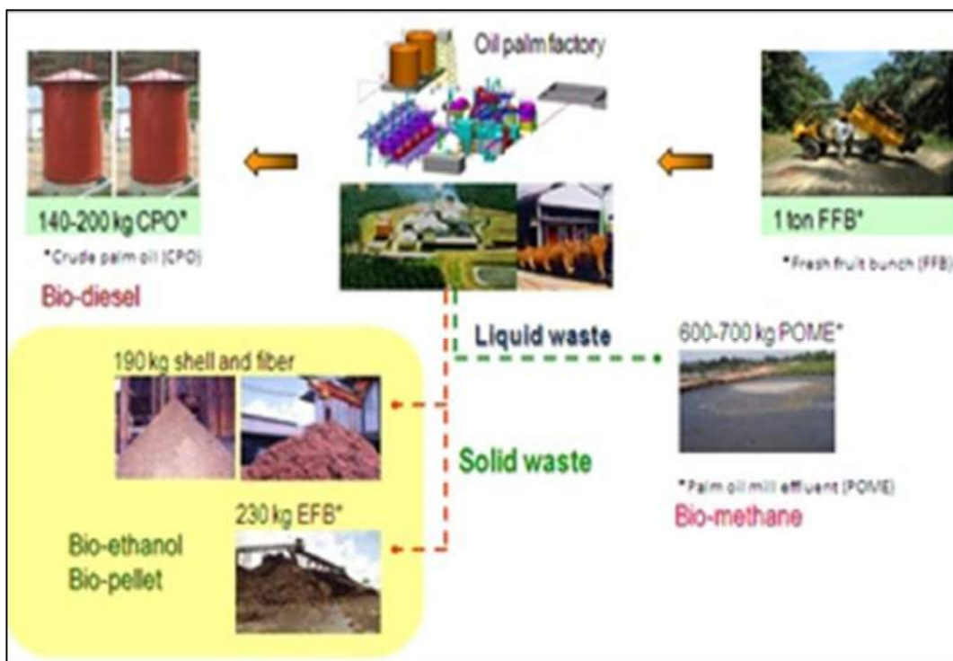
Figure 3.14 Mass Balance in palm oil processing industry (Kismanto, 2006 dimodifikasi: Aminta et al )
